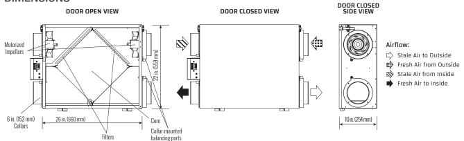
NOTE: Front clearance of 22 in. (559 mm) is recommended for servicing unit. All ducts use 6 in. (152 mm) round collars. MERV 13 upgrade: 485465 Weight: 42 lbs (19 KG) • Shipping weight: 44 lbs (20 KG)
