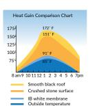
A white IB Roof Systems membrane can reduce your energy consumption and your rising electric bills, by reflecting up to 90% of the heat that normally enters a home through the roof. An IB Roof Systems roof will lower your home's heat gain, and possibly pay for itself.
